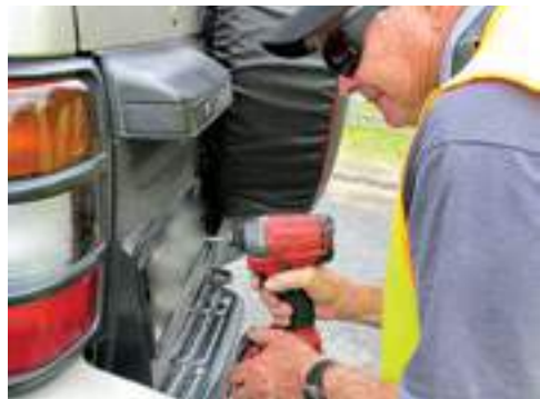
One-Way Security Screws make it almost impossible for number plates to be removed.
